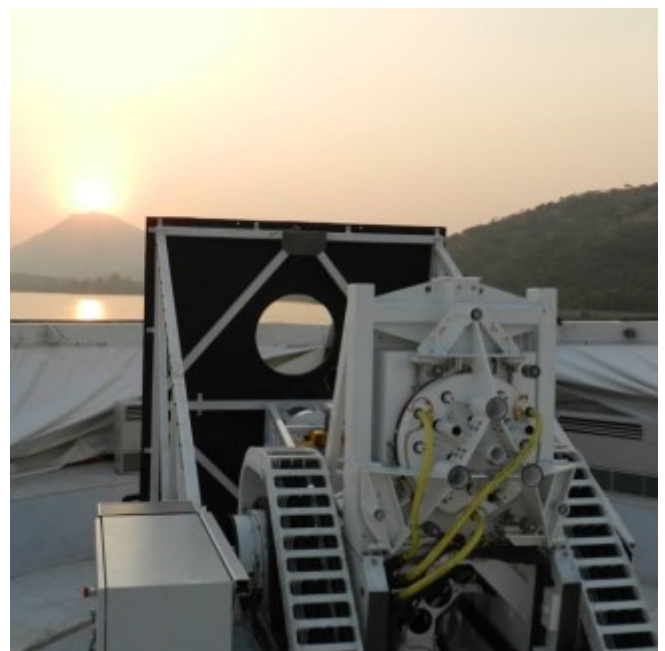
Figure 2. MAST pointing towards the Sun as the sun sets. The rear side of the primary mirror is seen here. The black plate with a circular opening is the sun-shield.
