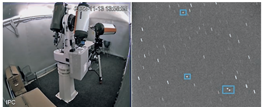
Figure 2: Noesis satellite-tracking sensor – a downscaled version of the current Holomondas system and surveying the EUTELSAT GEO slot.
