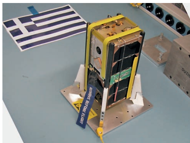
Figure 1: DUTHSat, a 2U CubeSat nano- satellite developed at DUTH, right before shipment for launch.
