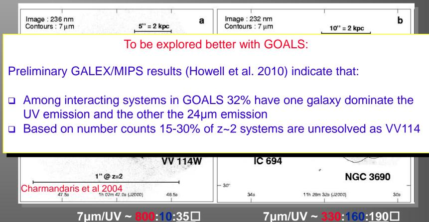
The spatial resolution of ground & Spitzer/MIPS24 surveys of LIRGs at z~2 will result in blending of the emission from the unresolved interacting components leading to a systematic underestimation of their dust content.
