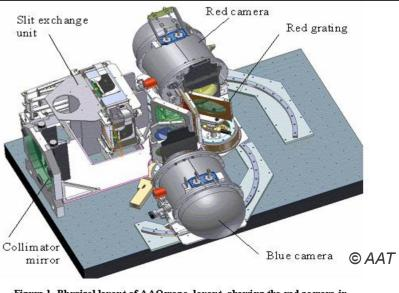
Figure 1. Physical layout of AAOmega, layout, showing the red camera in high dispersion mode, and blue camera in low dispersion mode.
