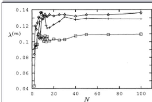
FIG. 4. The largest Lyapunov exponent as a function of  $N$  for  $\nu_c^{-1} = 0.8$  and  $\nu = 0.1$  (diamonds),  $\nu_c^{-1} = 0.8$  and  $\nu = 0.01$  (crosses),  $\nu_c^{-1} = 1.5$  and  $\nu = 0.1$  (squares). As in Fig. 3,  $\lambda^{(m)}$  is calculated for an integration time  $\tau = 30\ 000N$ , with time steps of  $\Delta\tau = 0.01$  and perturbations to the position and velocities of the blocks equal to  $10^{-5}$ .
