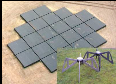
HBA tile-16 elements (3.5k E) Frequency coverage: 120 – 240 MHz
