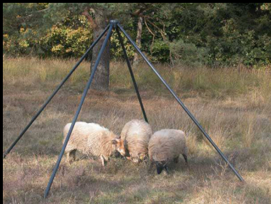
LBA (300E) Frequency coverage: 10 – 90 MHz (30 – 80) MHz
