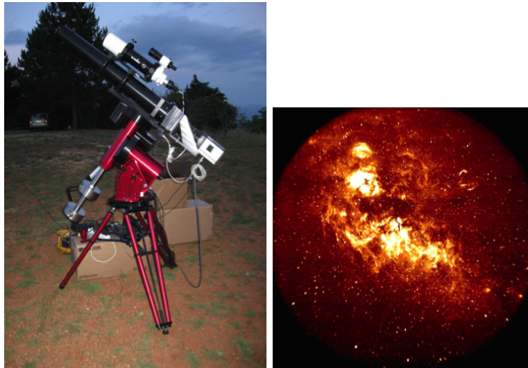
Figure 5: First light tests of MAWFC at the IAASARS Kryoneri Observatory. The instrument setup can be seen on the left image while on the right is the first light H \alpha image (20min exposure) in Cygnus.
