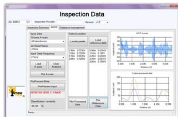
Human Machine Interface (HMI) developed for Non Destructive Evaluation applications. The presented HMI allows the automated defect detection, through Artificial Neural Networks, and hosts a defect recognition database which is automatically populated with inspection data.
