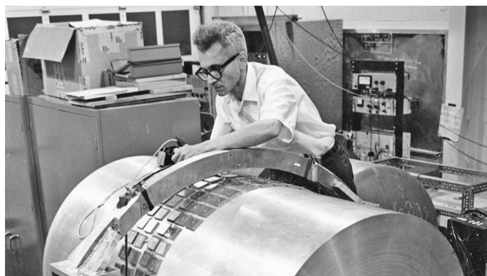
Figure 1: Joseph Weber working on the electronics of his bar detector.
