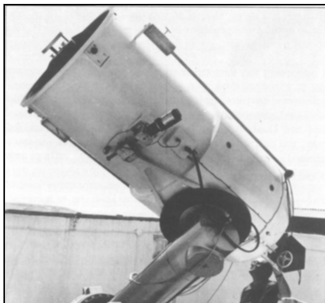
The 30-inch Cassegrain reflector of the Stephanion Observatory
