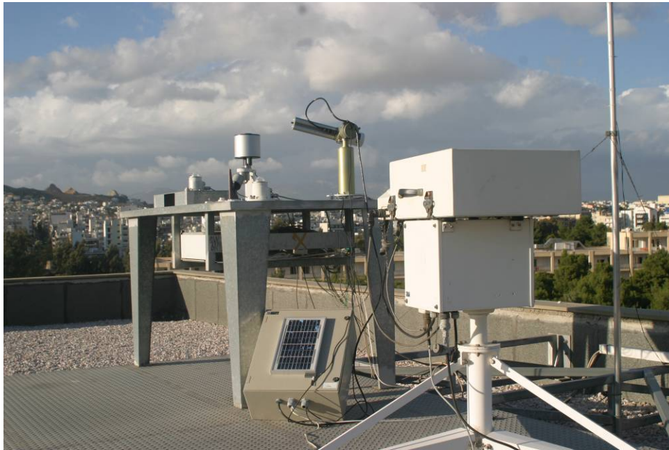
Figure 29: Aerosol sunphotometric station of ISARS will provide a long-term, continuous and readily accessible public domain database of aerosol optical, microphysical and radiative properties for aerosol research and characterization, validation of satellite retrievals, and synergism with other databases.
