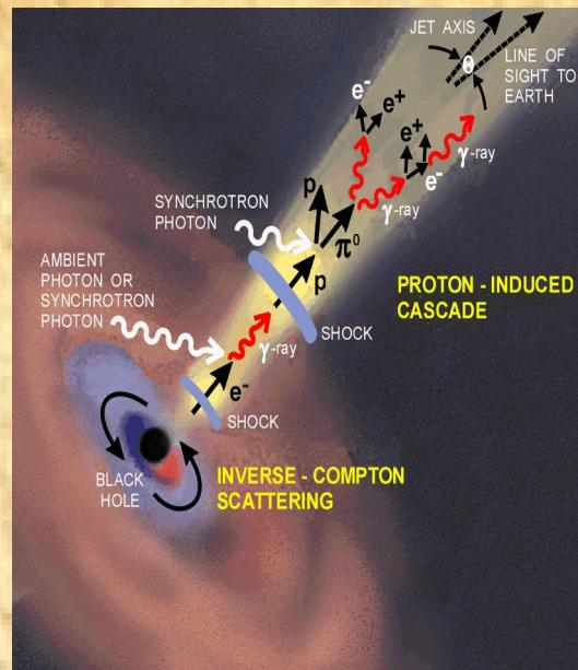
Inverse Compton scattering of synchrotron photons (SSC) or of external photons (ECS) by relativistic electrons
